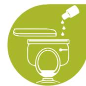
Put 15 drops of food colouring into the toilet cistern. If after 15 minutes the water in the toilet bowl has changed colour, there is a leak.
